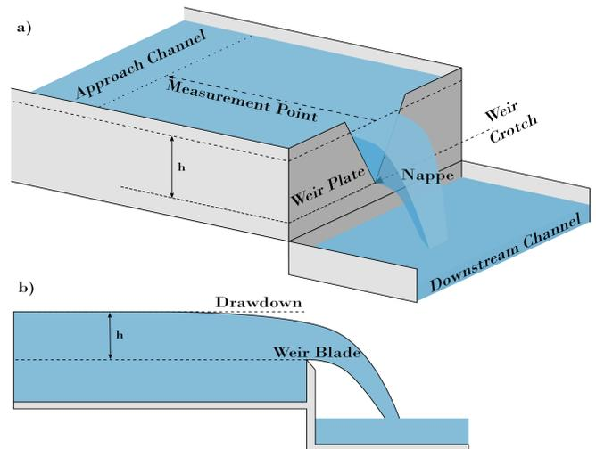
FIG. 1. a) A simple diagram of V-notch weir b) a cross section of the V-notch weir along its long axis. Several important parts of the weir have been labelled.
