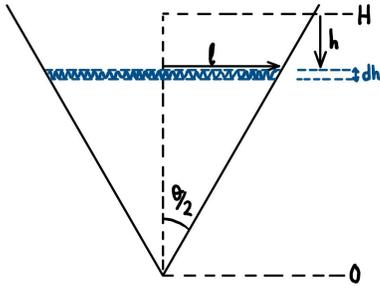
FIG. 2. The V-notch area broken up into slices of  $dh$  thickness.
